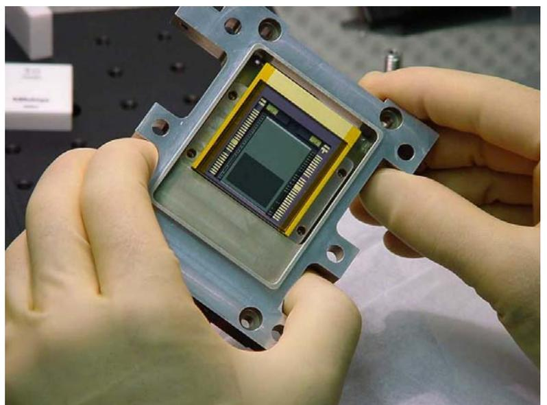
*OMI Detector Module seen from the CCD side.*
