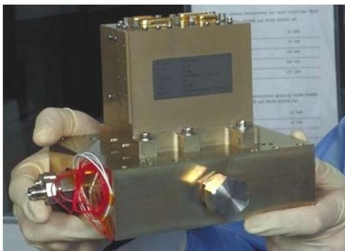
*The OMI Detector Module after the space qualification tests.*
