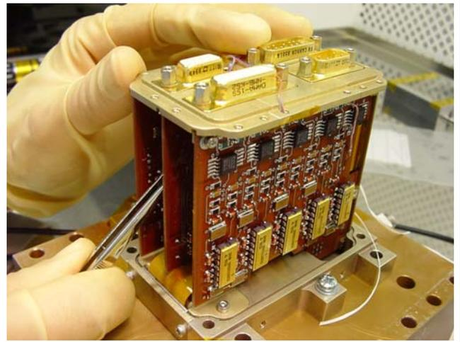
A view of the folded printed circuit board of the Detector Module during the integration.
