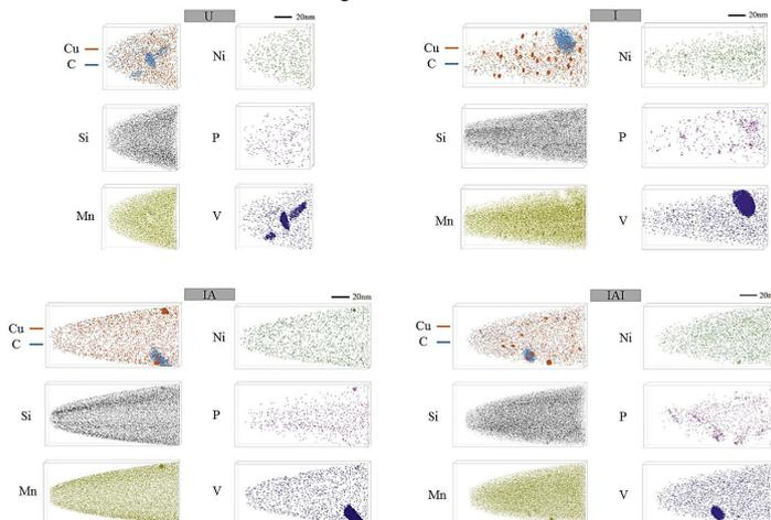
Figure 2. Typical atom maps of Cu, C, Si, Mn, Ni, P and V for model weld 501. [2]
