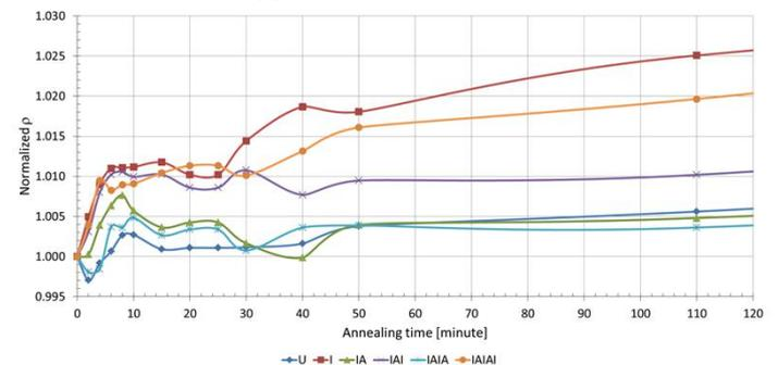
Figure 4. Electrical resistivity of model weld 501 as a function of annealing time in isothermal annealing at 420 °C. [4]
