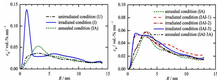
Figure 1. Size distribution of irradiation induced formations in model weld 501 measured by SANS. [1]
