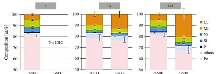
Figure 3. Composition of irradiation-induced defects measured by APT for a model weld 501. Average solute atom concentration in CRCs with less than 500 and more than 500 atoms. [2]
