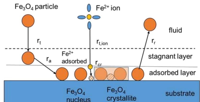
Figure 2. Scheme of the magnetite deposition process according to the proposed model.
