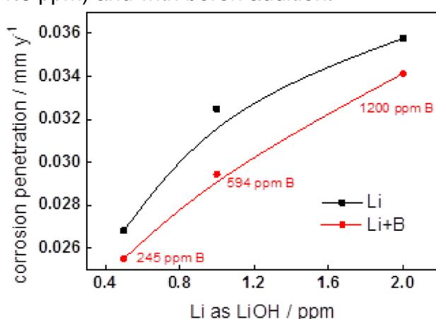
Figure 1. Corrosion penetration estimated from the oxidation rate constant  $k_1$  as depending on the water chemistry conditions during HFT. Alloy 690,  $T = 292^\circ\text{C}$ , exposure time 100 hrs, 1.3 mmol/l H<sub>2</sub> (= 30 cc/kgH<sub>2</sub>O).
