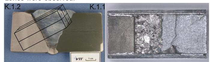
Figure 3. DMW mock-up, SE(B) specimens and resulting fracture surface.
