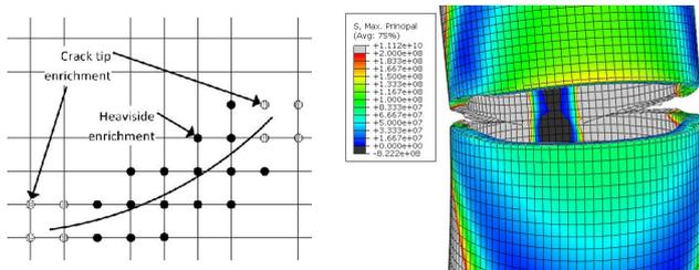
Figure 1. Left: Internal degrees of freedom that define the crack in XFEM analyses. Right: Crack growth path example from a pipe break analysis.
