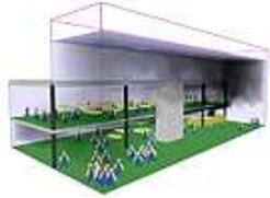
This is a fictitious atrium fire with 70 people on the first floor and 70 on the second floor. This example demonstrates the simultaneous simulation of fire and evacuation.
