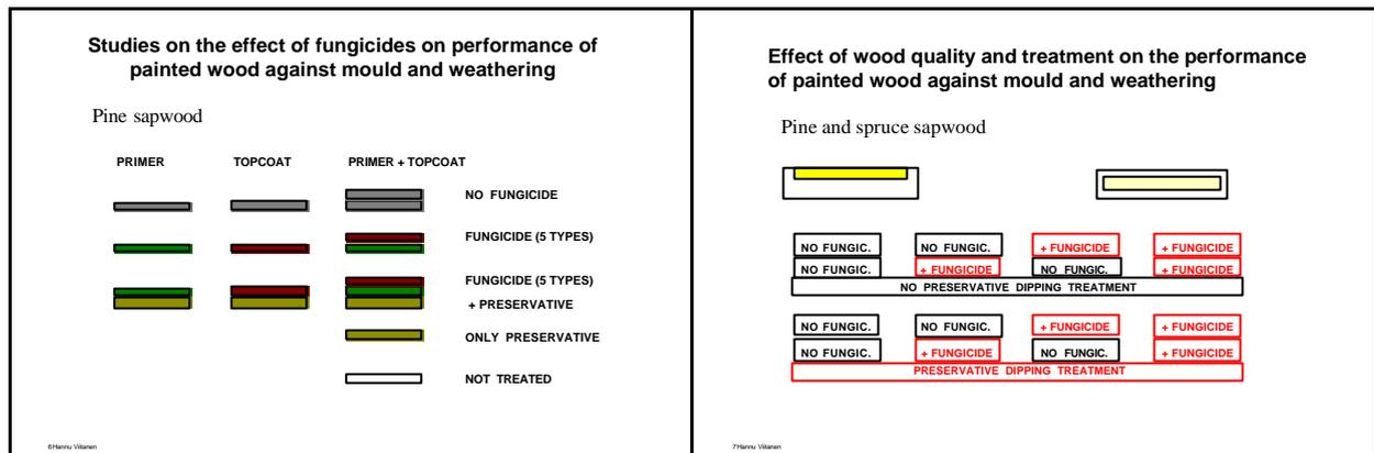
Figure 2. Different treatment systems for a) to study the effect of fungicides on pine sapwood and b) to study the effect of wood quality and treatment level on mould growth on pine and spruce sapwood.
