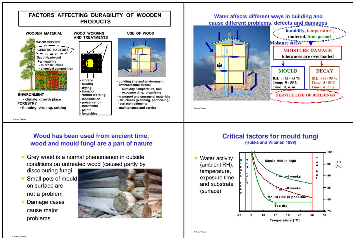
Figure 1. Factors affecting the durability of wood against mould and decay. Critical factors for the growth of mould fungi and the role of mould and bluestain fungi to produce grey wood.
