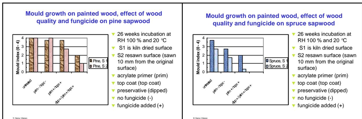
Figure 6. The mould growth on different painted pine (a) and spruce (b) sapwood after different treatment systems.
