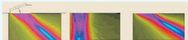
*Modelling of ultrasonic field. The fields shown in the figures are produced by a phased array ultrasonic transducer and demonstrate how the field can be directed using different delay laws for pulsing of the transducer elements.*
