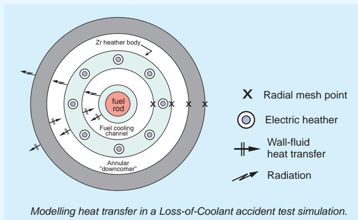
Modelling heat transfer in a Loss-of-Coolant accident test simulation.
