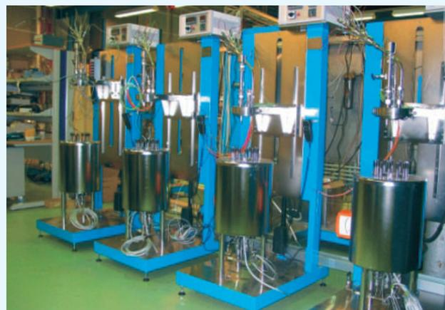
*Module autoclaves for corrosion fatigue life tests in LWR.*
