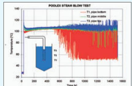
POOLEX test rig for steam blowdown experiments and a preliminary test result where oscillations inside the blowdown pipe are indicated by the temperatures measured at different elevations.
