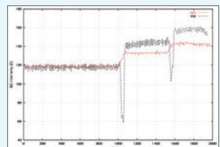
Calculated (APROS) and measured temperatures in the steam generators inlet in PACTEL experiment NCg-3.
