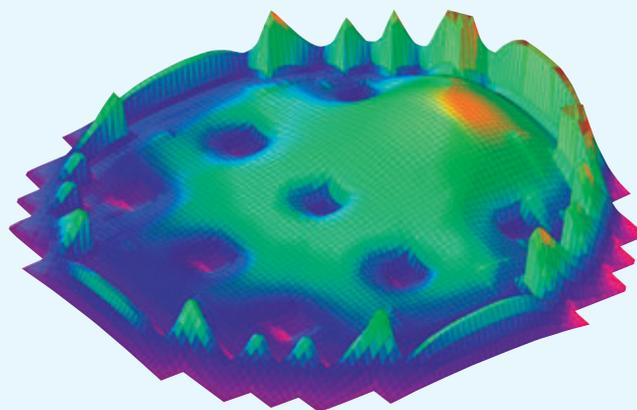
Thermal neutron flux in a PWR reactor calculated by the AFEN code.
