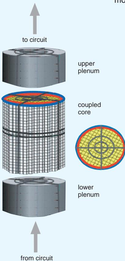
Internal coupling of reactor dynamics code TRAB-3D and thermal hydraulic code SMABRE.
