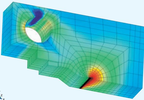
*Stress contours of a compact tension specimen finite element analysis model.*
