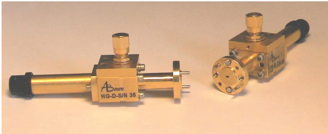
Figure 3. As an example of MVNA components: D-band (110 - 170 GHz, waveguide WR-6: 1.65 mm x 0.83 mm) source and detector. The detector is used also above 170 GHz. Waveguide test ports can be seen (without possible isolators etc. here now). Cables to MVNA main unit will be connected to top SMA connectors (which are shown here with static electricity protective short circuit terminations). Black adjusting knobs seen in the ends are for backshort tuning (useful for optimisation of operation).
