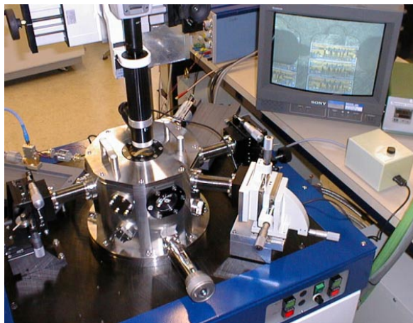
Figure 1. Cryogenic on-wafer measurement set-up at Millilab, VTT Information technology.
