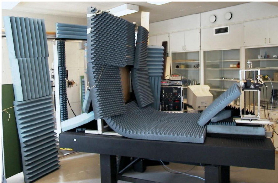
Figure 1. Measurement set-up for testing the quiet-zone at 310 GHz.
