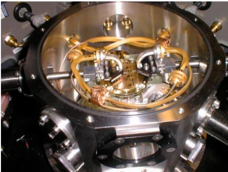
Figure 1. Cryogenic on-wafer measurement set-up
