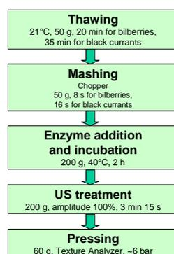
**Figure 1.** A schematic diagram of the juice extraction procedure investigated in this study.
