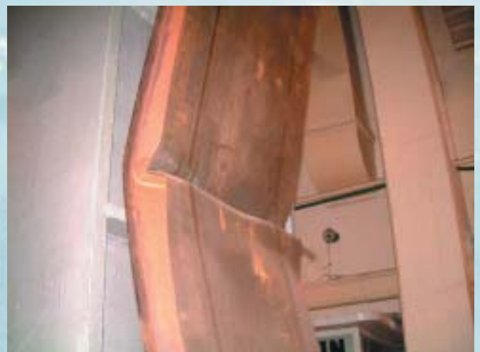
National KENNO research program: a panel after testing.
