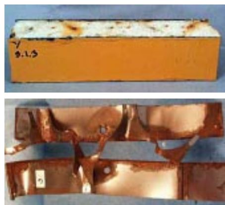
Fig. 5. The effect of PU foam on corrosion behaviour. The PU foam prevented corrosion except in the area near the specimen's edges.
