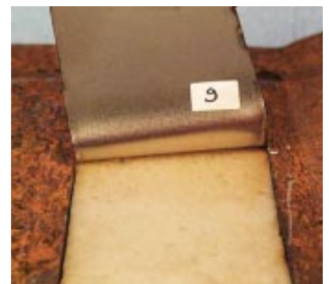
Fig. 4. An example of the specimen with stainless steel showing no visual corrosion even in the surface between cover and core plate (crevice corrosion).
