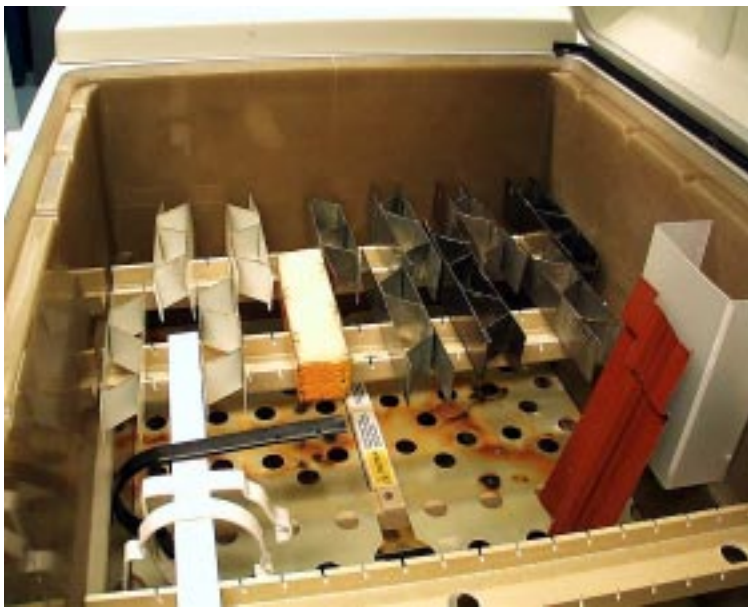
Fig. 1. Cyclic corrosion test box Q-Fog, model CCT and the test specimens inside the box.
