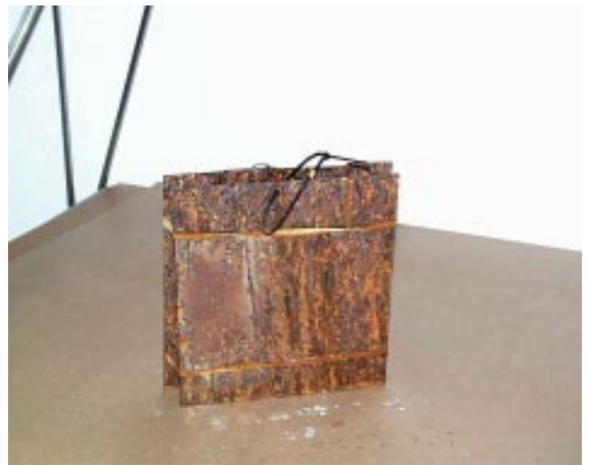
Fig. 2. An example of an uncoated specimen after corrosion testing.
