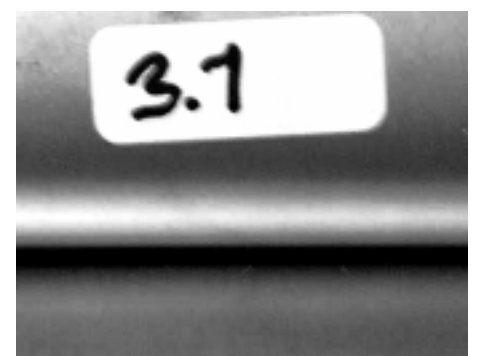
Fig. 4. An example of the specimen with stainless steel showing no visual corrosion even in the surface between cover and core plate (crevice corrosion).
