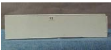
Fig. 3. An example of the specimen, after the corrosion tests, painted with typical paint used in ship wet spaces.
