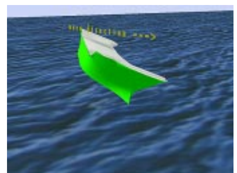
Fig. 1b. Visualisation of calculated ship motions in waves. Oblique stern waves, maximum roll angle. Wave direction is shown using 3-D text object above the ship.
