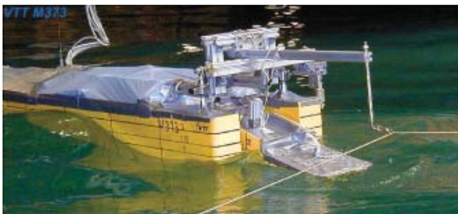
Figure 1. VTT carried out seaworthiness trial on five-metre models of ATB combinations.
