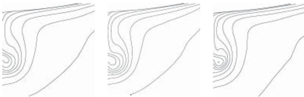
Figure 1. Computed wakes at the propeller plane. From the left to the right: Chien's low-Reynolds number  $k$ - $\epsilon$  turbulence model, Chien's low-Reynolds number  $k$ - $\epsilon$  turbulence model with Menter's modification for the turbulent viscosity, Menter's SST  $k$ - $\omega$  turbulence model.
