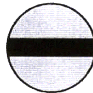
(iv) 'Sandwich' type fibre
